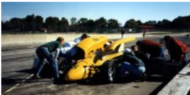
Raider Lightning crew changing batteries during a pit stop.
