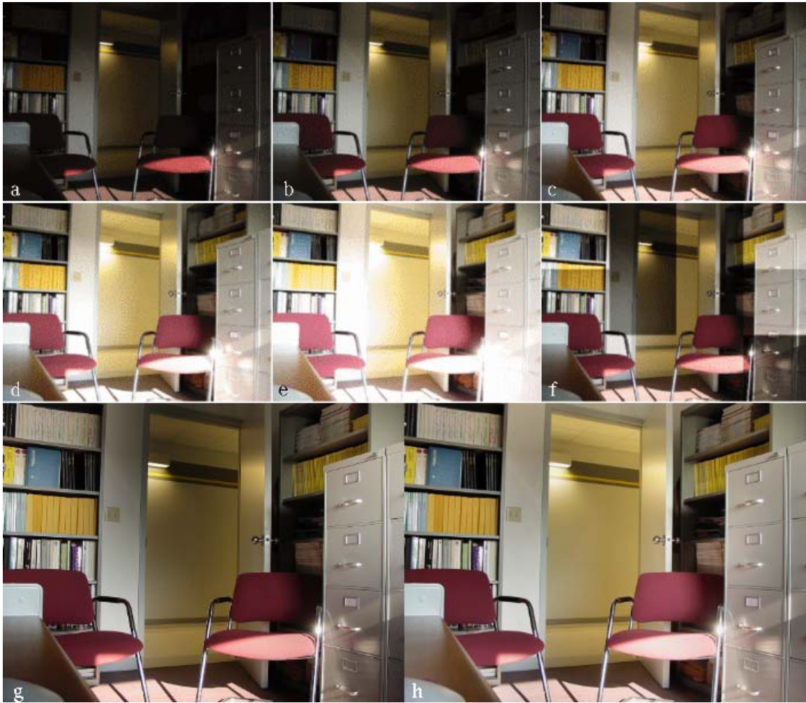
Figure 1: (a)–(e) Images representing different exposures of an office room. (f) The image obtained by composing the twelve subimages (image blocks) cut out of the five images. (g) The image produced by centering the blending functions at the selected blocks in the images, multiplying the blending functions with image colors, and adding the weighted colors together. (h) The most informative image constructed from images (a)–(e).
