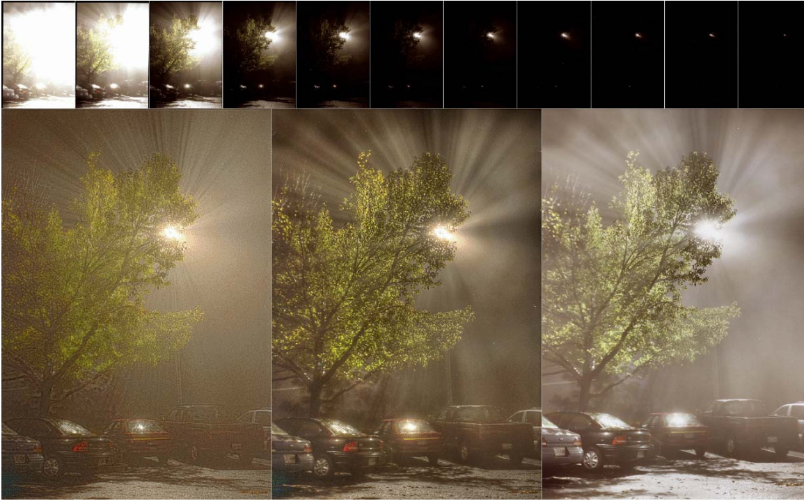
Figure 6: The top row shows eleven original images, and the images below that from left to right show the results obtained by the methods of Tumblin and Turk, and Fattal et al., as well as our method. The original images are courtesy of Jack Tumblin.
