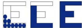
(a) Raster scan writing scheme; (b) vector scan writing schemes; and (c) shapes of electron beam: round, variable, cell projection.
