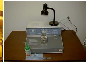
Critical Point CO 2 Dryer 31 °C and 7.38 MPa
