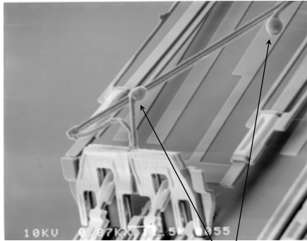
“Burned out” electro-thermal actuator hot arm
