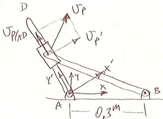
$$\omega_A = 10 \frac{\text{RAD}}{\text{s}} \rightarrow, \alpha_A = 0$$
