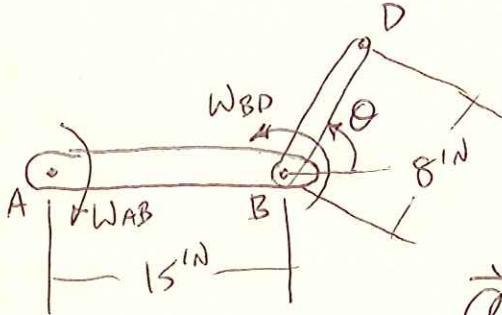
$$\omega_{AB} = 5 \frac{\text{rad}}{\text{s}} \rightarrow, \omega_{BD} = 3 \frac{\text{rad}}{\text{s}} \rightarrow$$
