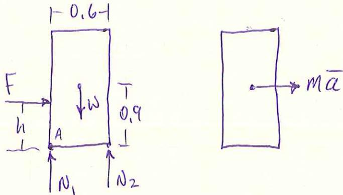
$$W = mg = (20 \text{ kg}) \left( 9.81 \frac{\text{m}}{\text{s}^2} \right) = 196.2 \text{ N}$$
