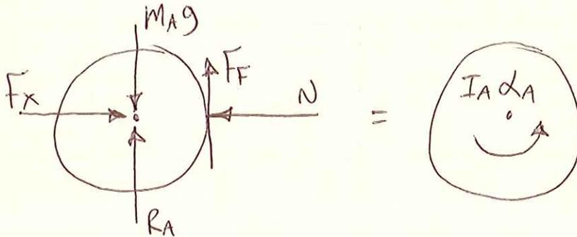
$\sum \vec{M}_G = \sum (\vec{M}_G)_{\text{EFF}} + \curvearrowright: r_A F_f = I_A \alpha_A$
