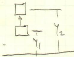
WORK OF A GRAVITY FORCE ONLY DEPENDS ON THE INITIAL AND FINAL ELEVATIONS.
