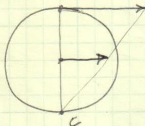
WHICH YOU CAN ASSUME A BODY IS ROTATING AT A GIVEN INSTANT. THIS CAN BE USED TO FIND  $\omega$  OR VELOCITIES ON THE BODY.
