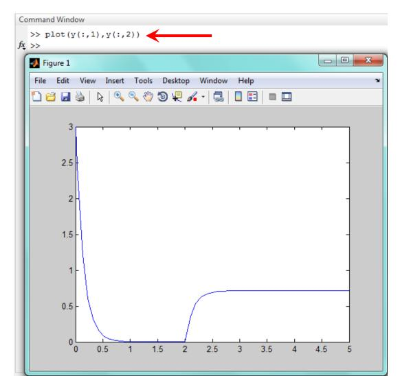
You can publish the Simulink model and the results by creating a MATLAB Script file that calls it. First, close the Simulink model. The name of the Script file must be different than the Simulink model. Open the Script file and use the Publish function.
