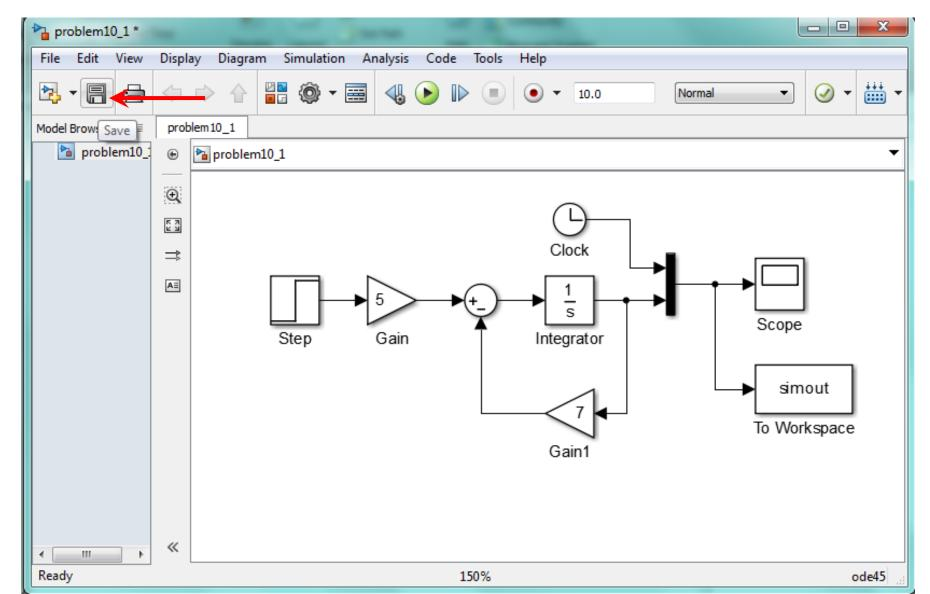
Change the Run Time to 5 sec and Run the model. Wait for the Ding! Double-click on the Scope block to plot the output.
