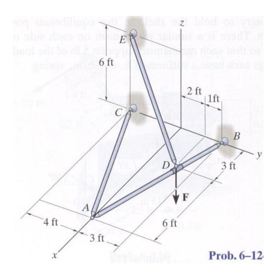
4. (20 points) Draw **all** of the necessary the free-body diagrams for the following situations. Do not solve!
