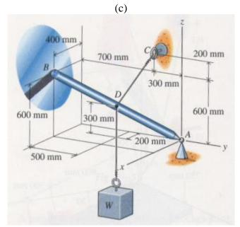
The block *W* has a mass of 250 kg. Bar *AB* rests against a smooth vertical wall at end *B* and is supported at end *A* with a ball-and-socket joint. The two cables are attached to a point on the bar midway between the ends. Determine the reactions at supports *A* and *B* and the tension in cable *CD*.
