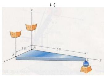
The triangular plate of uniform thickness shown weighs 750 lb. Determine the tensions in the two cables supporting the plate and the reaction at the ball support.
