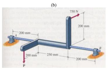
The shaft with two levers is used to change the direction of a force. Determine the force **P** required for equilibrium and the reactions at supports A and B. The support at A is a ball bearing and the support at B is a thrust bearing. The bearings exert only force reactions on the shaft.
