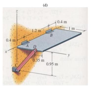
The door shown has a mass of 25 kg and is supported in a horizontal position by two hinges and a bar. The
