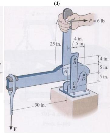
If a force of P = 6 lb is applied perpendicular to the handle of the mechanism, determine the magnitude of force *F* for equilibrium. The members are pinconnected at *A*, *B*, *C*, and *D*.
