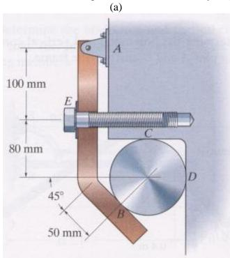
The link is used to hold the rod in place. Determine the required axial force on the screw at E if the largest force to be exerted on the rod at B, C, or D is to be 100 N. Also, find the magnitude of the reaction force at pin A. Assume all surfaces of contact are smooth.
