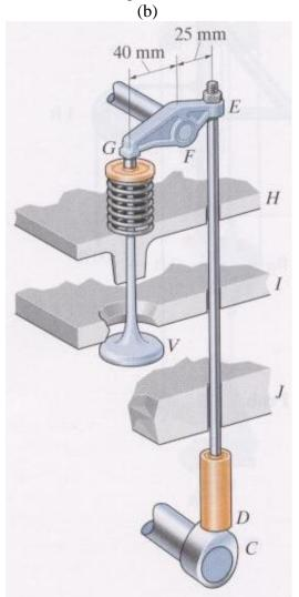
Operation of exhaust and intake valves in an automobile engine consists of the cam C, push rod DE, rocker arm EFG which rides on a smooth bearing at F, and a spring and valve, V. If the compression in the spring is 20 mm when the valve is open as shown, determine the normal force acting on the cam lobe at C. Assume the contact between the cam and the push rod at D is normal and smooth. The spring has a stiffness of 300 N/m.
