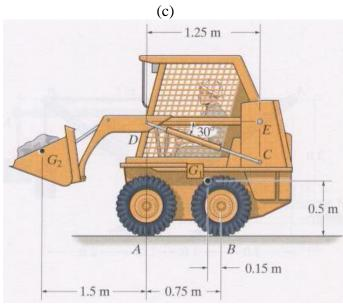
The skid steer loader has a mass of 1180 kg, and in the position shown the center of mass is at  $G_1$ . If there is a 300-kg stone in the bucket, with center of mass at  $G_2$ , determine the reactions of each pair of wheels A and B on the ground and the force in the hydraulic cylinder CD and at the pin E. There is a similar linkage on each side of the loader.
