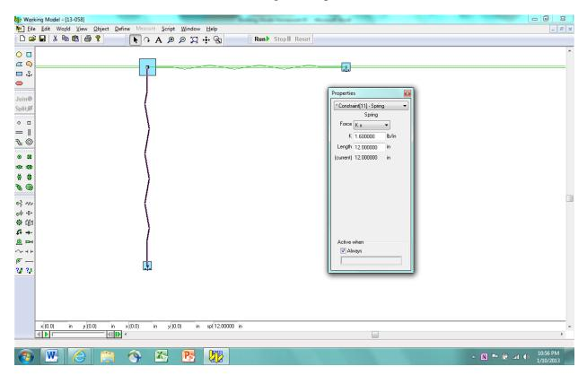
Move the block to x = 5.0 inches, thereby compressing the horizontal spring. Use the type-in boxes to set the value of the location to exactly x = 5.0 inches.
