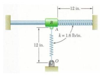
Open Working Model. Go to the View Tab/Numbers-and-Units and change the Unit System to English (pounds). Create a 10-lb block and locate it at x = 0 and y = 0. Use the Horizontal Keyed Slot Joint at the center of the block. Place and anchor small blocks at point *O* and to the right of point *A* as shown below.
