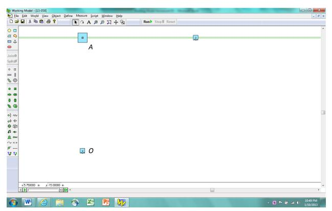
Use the Spring Tool and place springs as shown below. Change the spring constant of the springs using the Properties Window for each spring. Note that the spring force is defaulted to be F = kx, but other nonlinear choices can be made using the drop-down menu.
