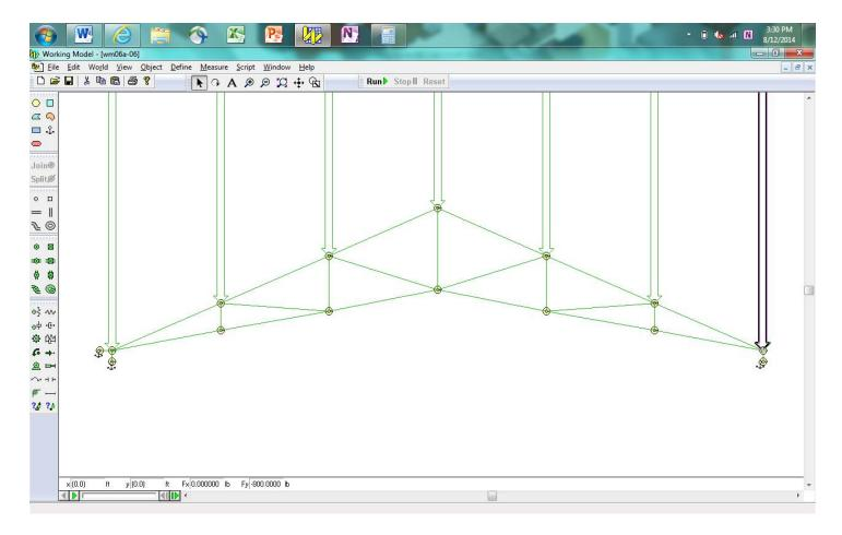
Place force measurement output boxes on the external reaction rods and the requested rods within the structure. Run the simulation to obtain the solution.
