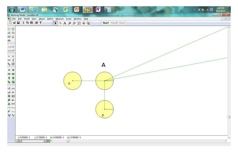
Since point L is supported by a roller bearing, which only supports normal loads, connect point L with a rod as shown.
