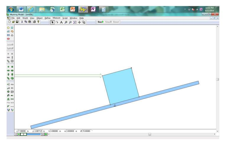
Run the simulation iteratively to determine the force required for the block to move. Then iteratively determine the static friction coefficient for the block to slide instead of tip.
