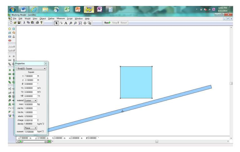
Change the static and kinetic coefficients of friction of the touching surfaces by double-clicking and bringing up the Properties dialog boxes. Initially, set the static coefficient of friction to 1.0. Run the simulation so that the block falls onto the base. Then use World/Start Here to reset the simulation to the new point.
