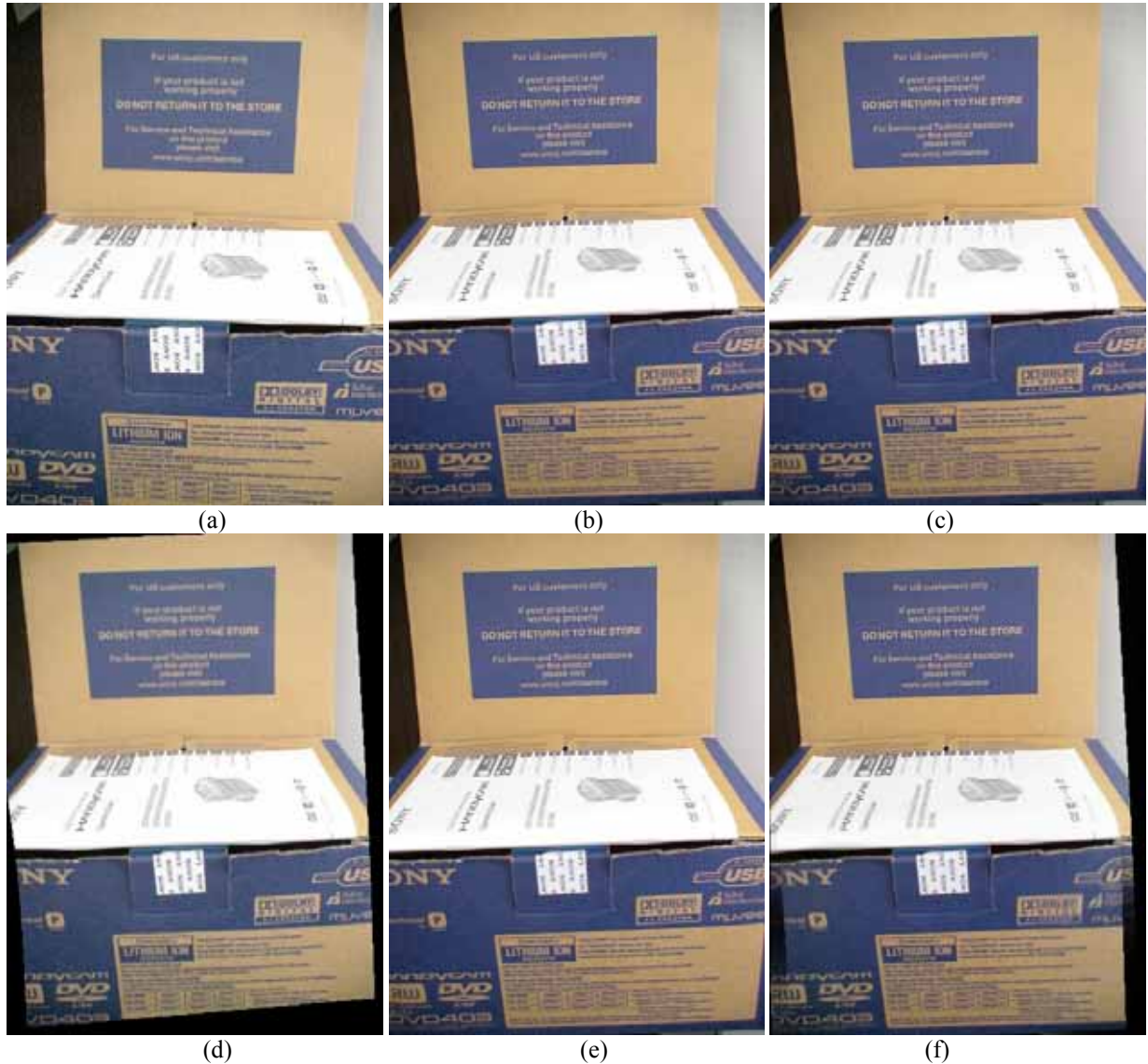
Figure 4. (a)–(c) Images of a box scene obtained by focusing the camera on the bottom, the middle, and the top planes. (d), (e) Warping images (a) and (c) to the geometry of image (b). (f) Fusion of images (b), (d), and (e).
