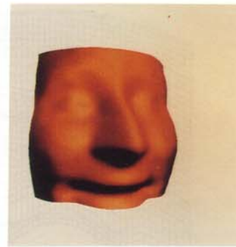
Colour Plate 10 Approximation of wireframe shown in Figure 11 by a RaG surface [Each grid point was used as a control point.]
