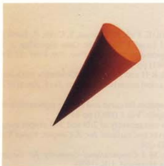
Colour Plate 8 Cylinder; (a) cylinder obtained by interpolating half-closed RaG surface to vertices of two equal and parallel equilateral triangles, (b) when area of one triangle approaches zero, cylinder is transformed to cone
