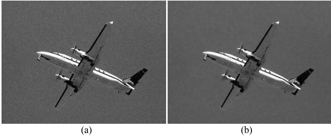
Fig. 12. (a) Zero-mean uniformly distributed noise corrupting the image of a plane. (b) Adaptive Gaussian filtering with \sigma_x = a/2(g_n+1) and \sigma_y = a/2(g_m+1) , where g_n and g_m are the minimum and maximum gradient magnitudes at a pixel and a = 6 pixels.
