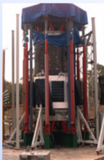
8-ft composite LH2 tank, X-33
