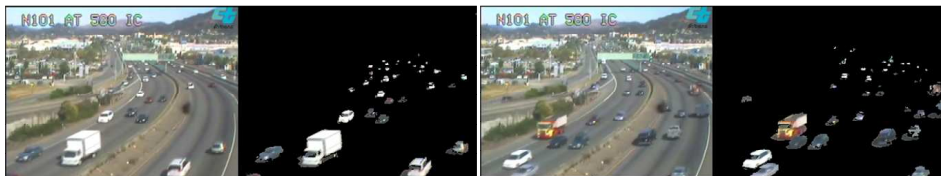
Figure 3: Performance of SILK on a road traffic sequence (moving car detection) task, with a jittery camera. Two random frames and the performance of SILK on those frames are depicted.
